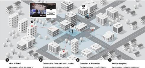
When a gun is fired, the sound of a muzzle blast radiates outward. Acoustic sensors are triggered by the impulsive sound. The sound is classified as a gunshot using artificial intelligence and triangulation determines the precise location. e data is relayed to the ShotSpotter ident Review Center where analysts ickly audit the data and publish for immediate infirmed gunshots to police.
